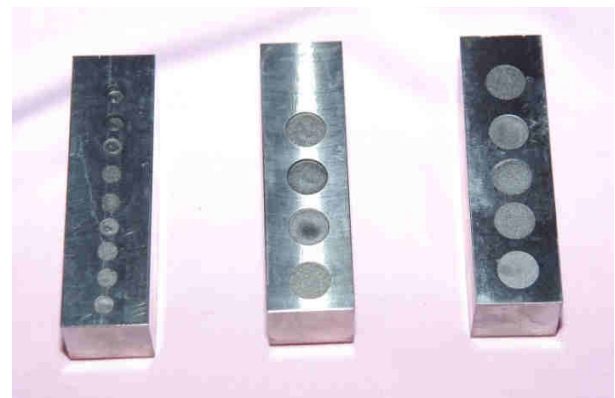
Fig. 2. Ti-6Al-4V workpiece after EDM machining.
